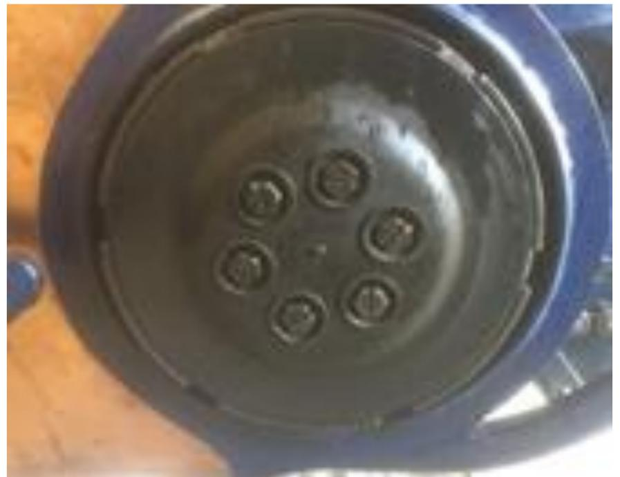
**The assembled Jardine Multiplate Clutch showing the outer plain disc and retaining bolts.**
