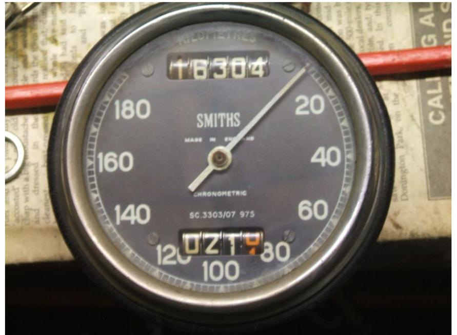
Smiths' speedos and tachos have a code which identifies the style of the instrument and, often, what it was used on. While I'm quite happy playing around with magnetos and dynamos getting the needle off its spindle without damaging it or the dial is not easy. SC.3303/07 975 is the kilometers per hour equivalent of a 120mph speedo intended for BSA 500 pre-unit singles.
