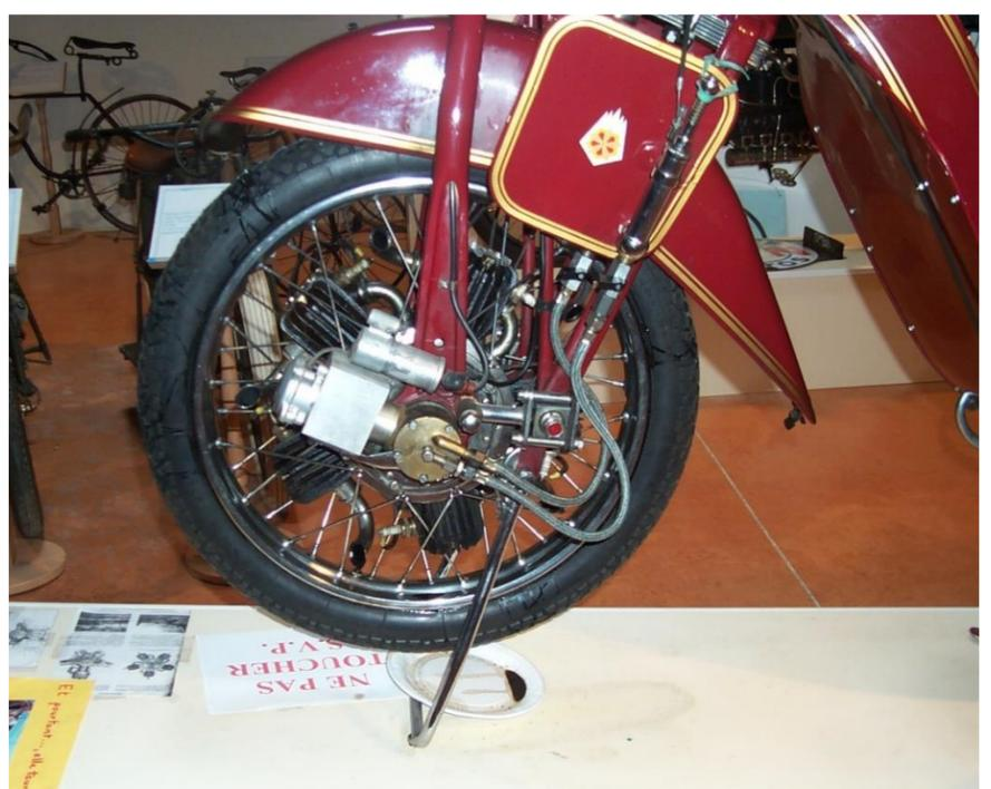
Views from either side looking directly at the engine, these shots show how the carburettor, sparks and oil pass through the front wheel spindle to the spinning engine. According to Erwin Tragatsch, they were manufactured in Munich from 1921 through to 1925 and were said to have first class roadholding!
