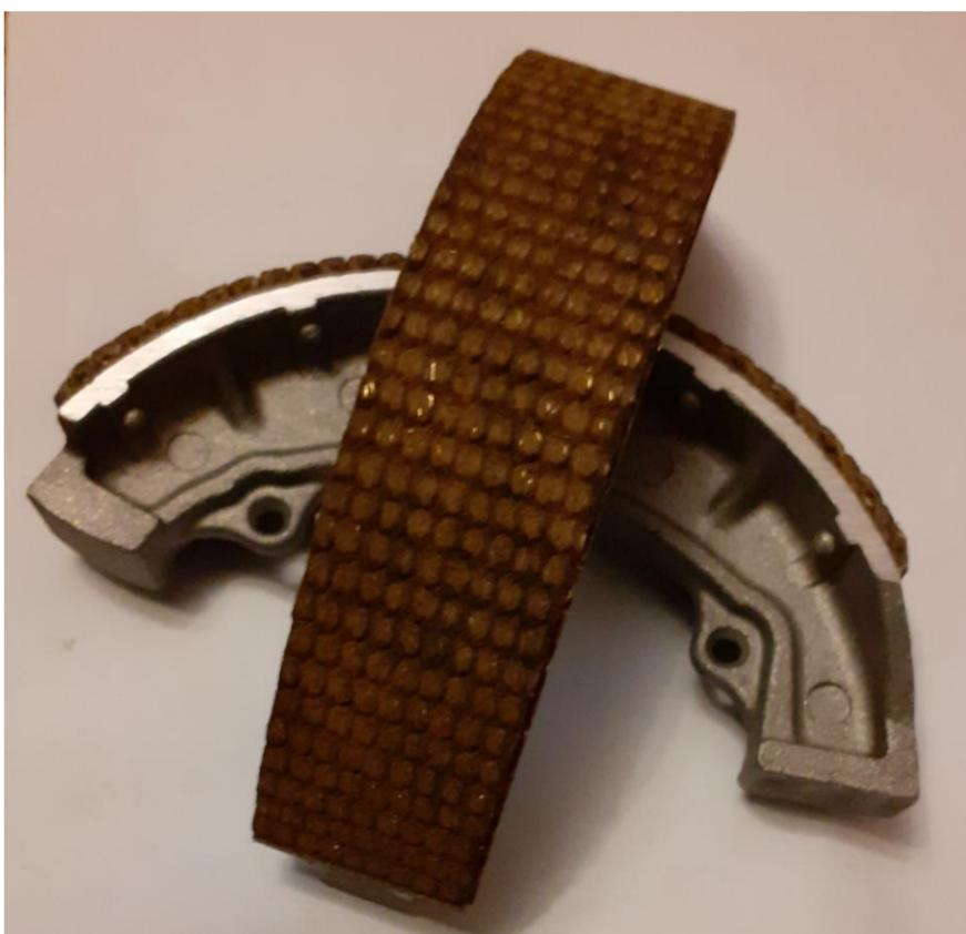
Shoes for the twin-leading shoe front brake on my 1969 Tiger 100, freshly re-lined by Villiers Services. I opted for bonded rather than the original riveted linings because my experience with this woven material used by Villiers Services is that it provides excellent stopping power. Good value at less than £30/pair including p&p. New replacement shoes aren't available for the 7-inch TLS Triumph brake, just the 8-inch - and they would be a bit of a tight squeeze.
