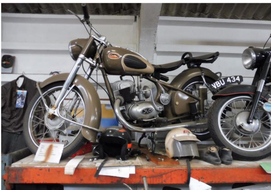
**I think this is a 1950s Radex Express, built in Germany, using an ILO engine (stylised as JLO on the crankcase) – the information on the card was obscured by the rust stain from the forks!**
