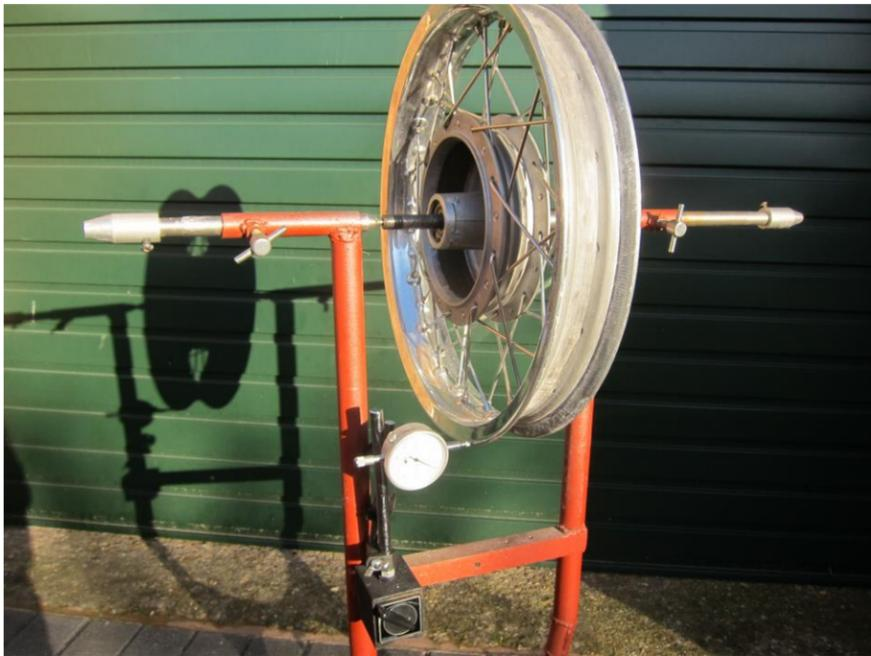
**Photo 2 – Doing likewise with the lateral run out**
