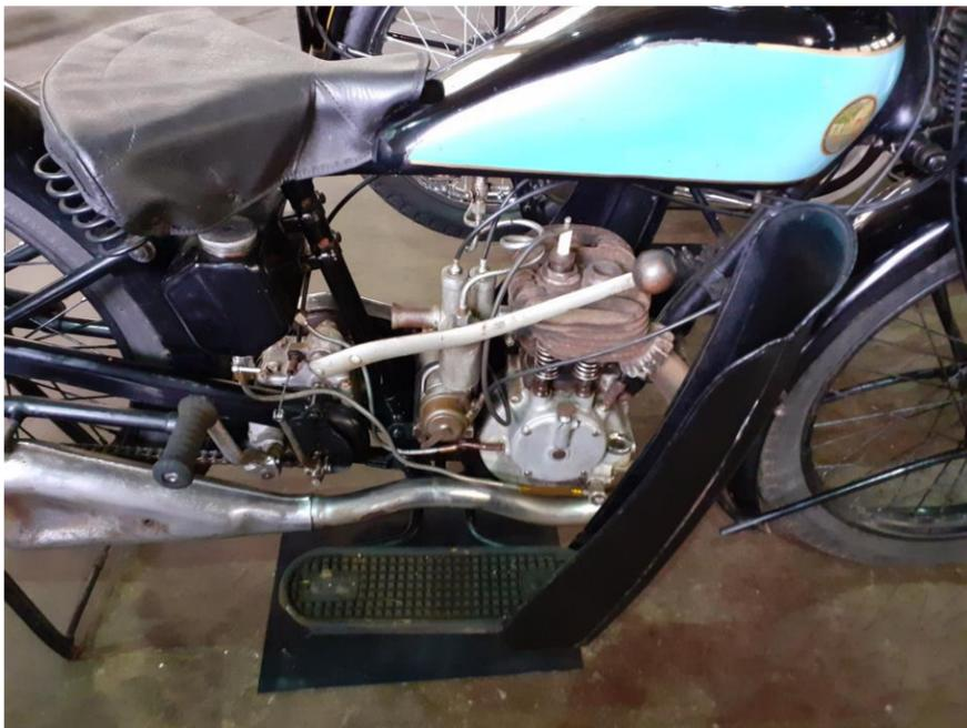
The “power plant” and three-speed gearbox
