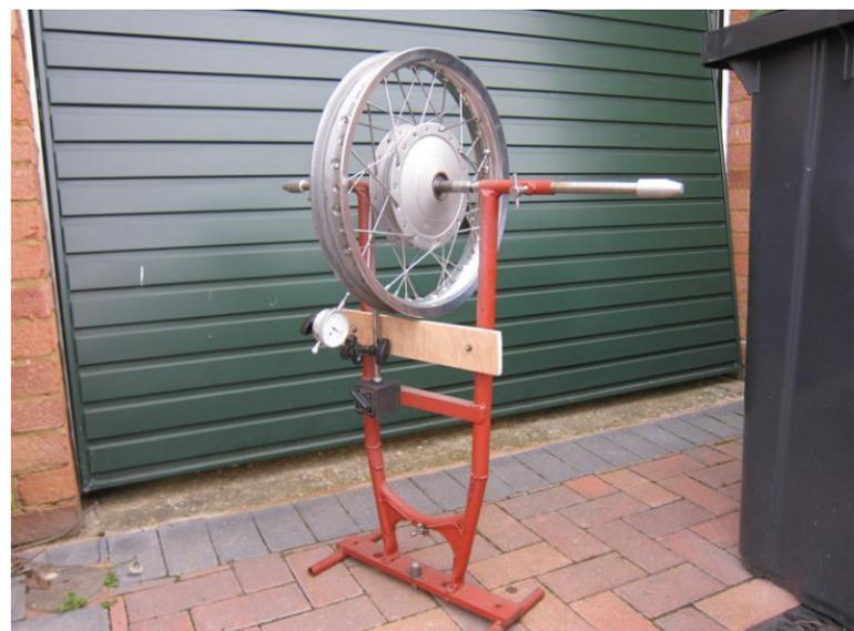
Photo 1 - Sorting the radial run out with the dial gauge
