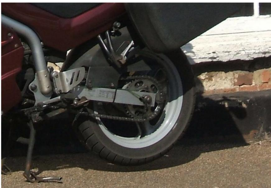
New chain, sprockets and Scottolier - It can't have been that difficult, can it?
