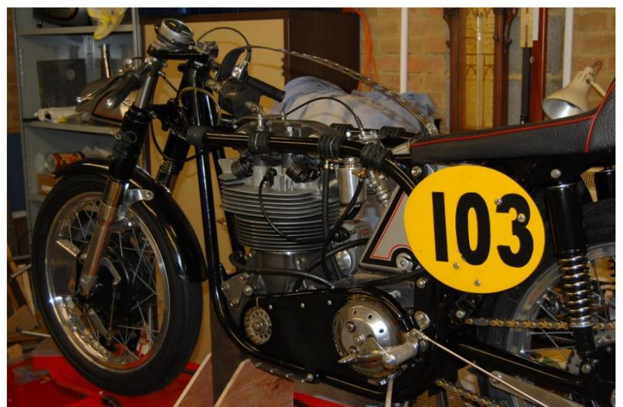
The Manx without fuel tank and front nose cone, undergoing maintenance as is very usual between races. Note how tall the engine is in the frame.
