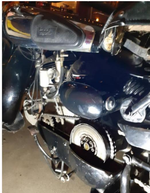
The SS80 clutch exposed and partially dismantled
