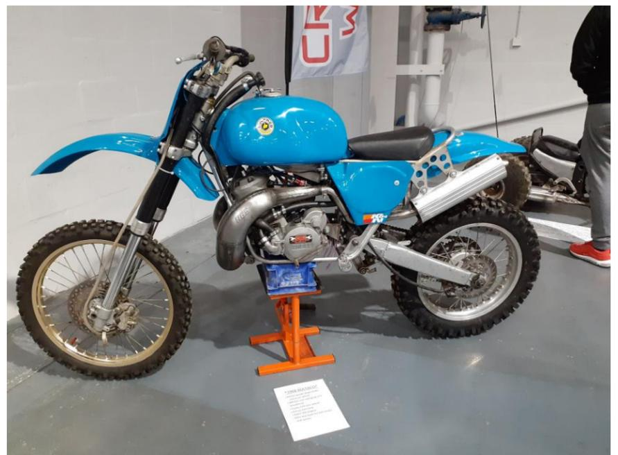
"Bultaco" built for hill-climbs and sprints - using KX 250 forks, WR200 swing-arm, Husky rear wheel, Ducati fuel tank, 700 Zabel engine
