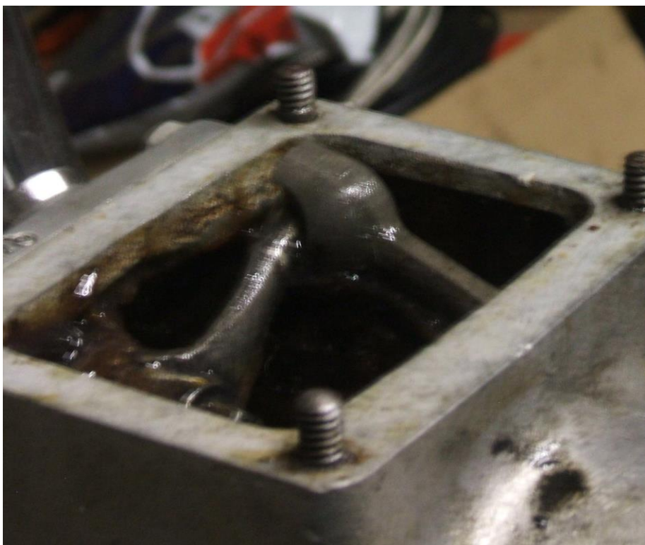
Not much to see really. The hole in the trunnion fits over the end of the arm on the left and the trunnion fits into the spherical end of the arm on the right.
