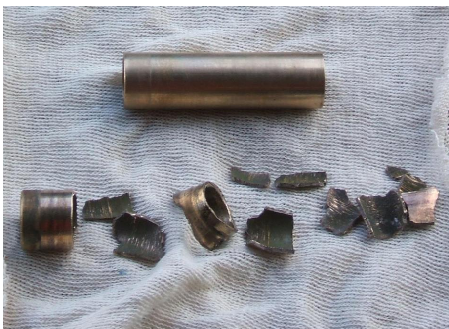
At the top is the replacement bush. What's left isn't much good as a pattern
