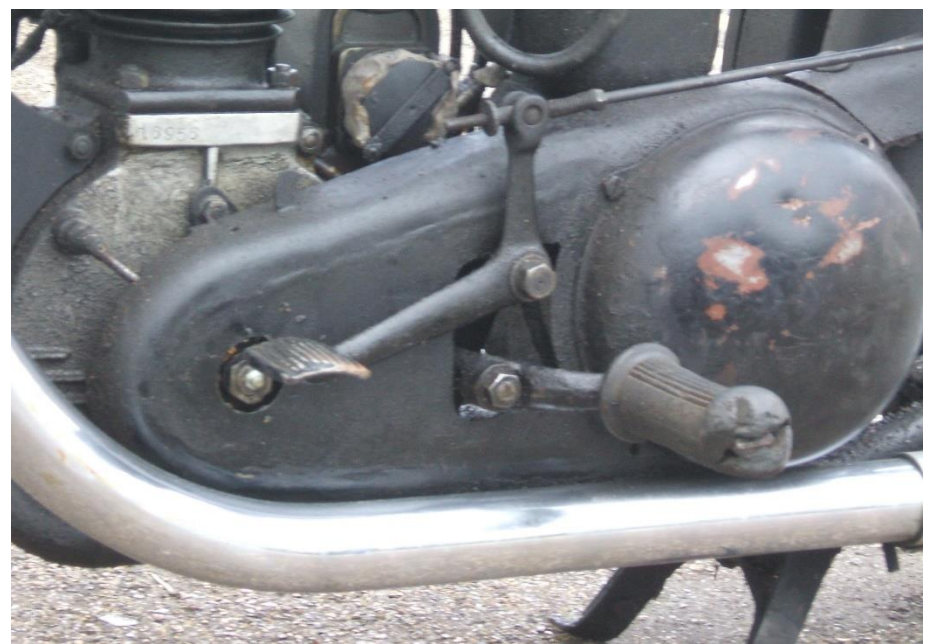
Primary chain guard with the clutch cover - 'bowler hat' - behind the footrest
