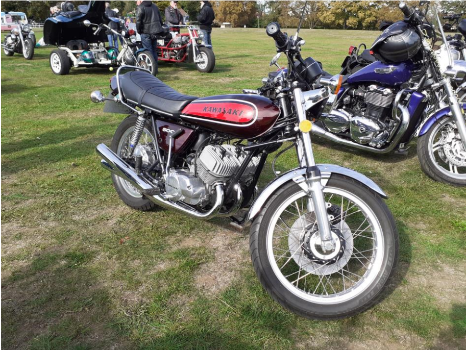
“Widow-maker” Kawasaki two-stroke triple – here in 500cc guise but 400cc and 750cc models were also present.
