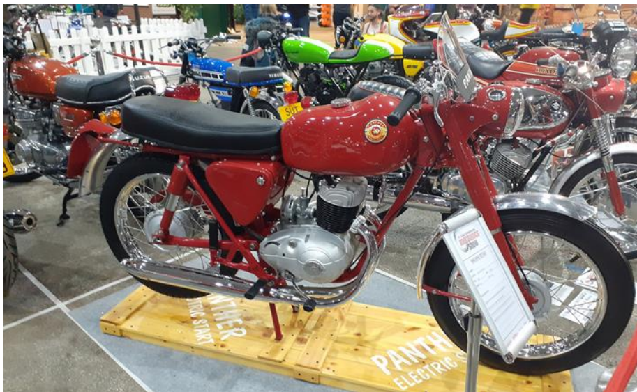
The dying gasp of a once proud cat – the last of the Panther 250s, using up Villiers 2T dynastart engines from a cancelled microcar order
