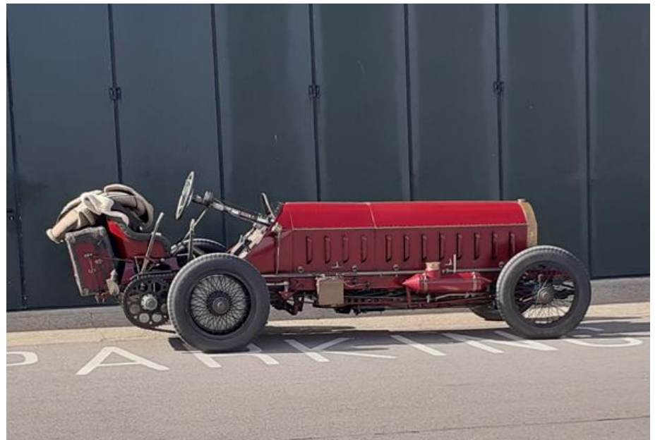
1903 or 4 Fiat, with an engine from an airship
