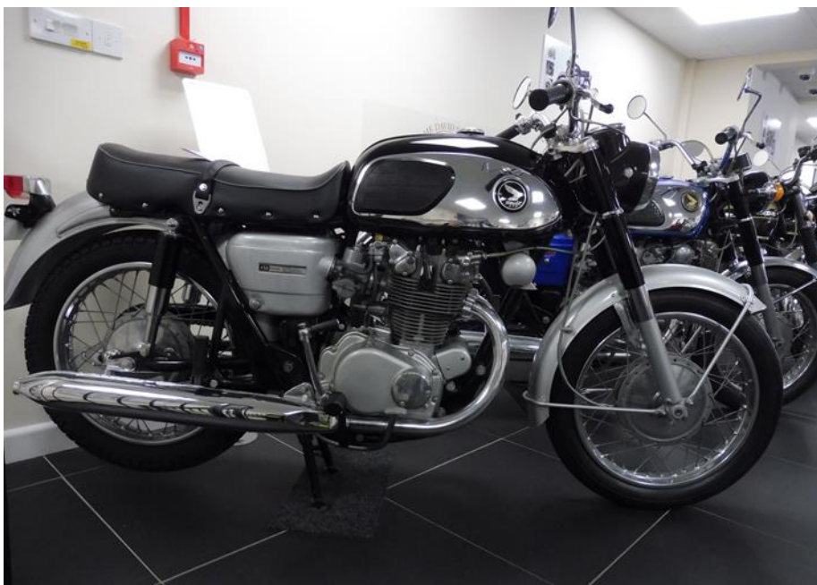
1965 Dream CB450K0 “Black Bomber” – 444cc, 43bhp at 8500rpm, twin-cylinder, twin 32mm CV carburetors and twin leading-shoe front brake. Honda’s first large capacity machine. The bike in the collection is an early American production model with zero miles on the clock.
