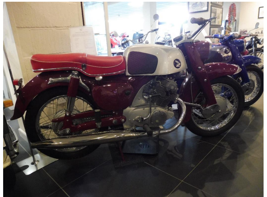
1959 Dream CE71 Super Sport – electric start, 250cc twin-cylinder OHC. The follow-up to the C71 released the previous year. Intended primarily for the American market, only 390 bikes are believed to have been produced. It's rumoured that, for reasons unknown, Honda tried to buy them all back. This is possibly the rarest of all production Hondas.
