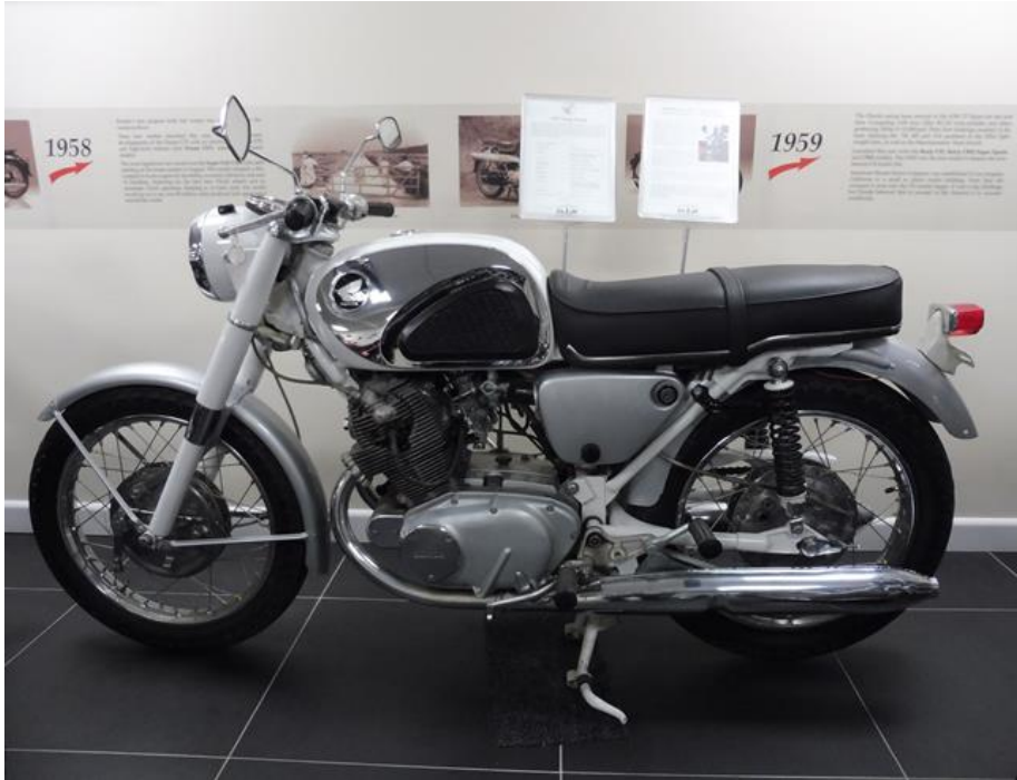
1964 CB77 Super Hawk – 305cc, twin-cylinder, twin carbs; first introduced in 1961 and produced until 1968. Elvis Prestley rode one of these in the 1964 film “Roustabout”. The example in the collection has only 283 miles on the clock since its restoration.
