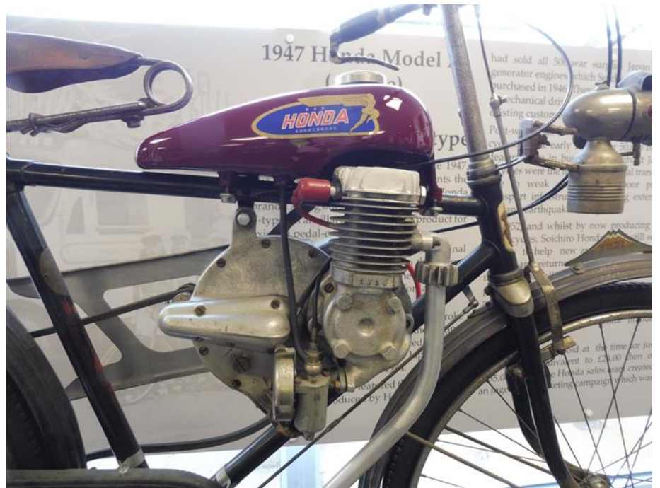
Close-up of that 1hp clip-on engine and petrol tank
