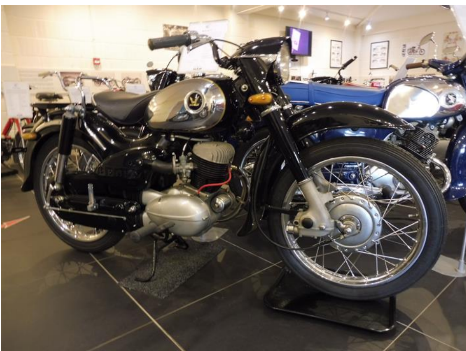
1957 125cc Benly JC-57 – originally introduced in 1956 but now with increased power, fully enclosed rear chain and oil-damped bottom-link suspension replacing the previous earles-fork type.
