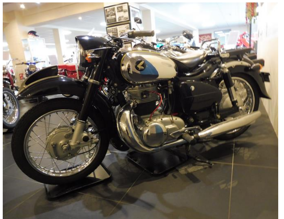
1956 Dream MF - 345cc, four-speed, single-cylinder OHC four-stroke. 20bhp at 6500rpm. One of only five known survivors.
