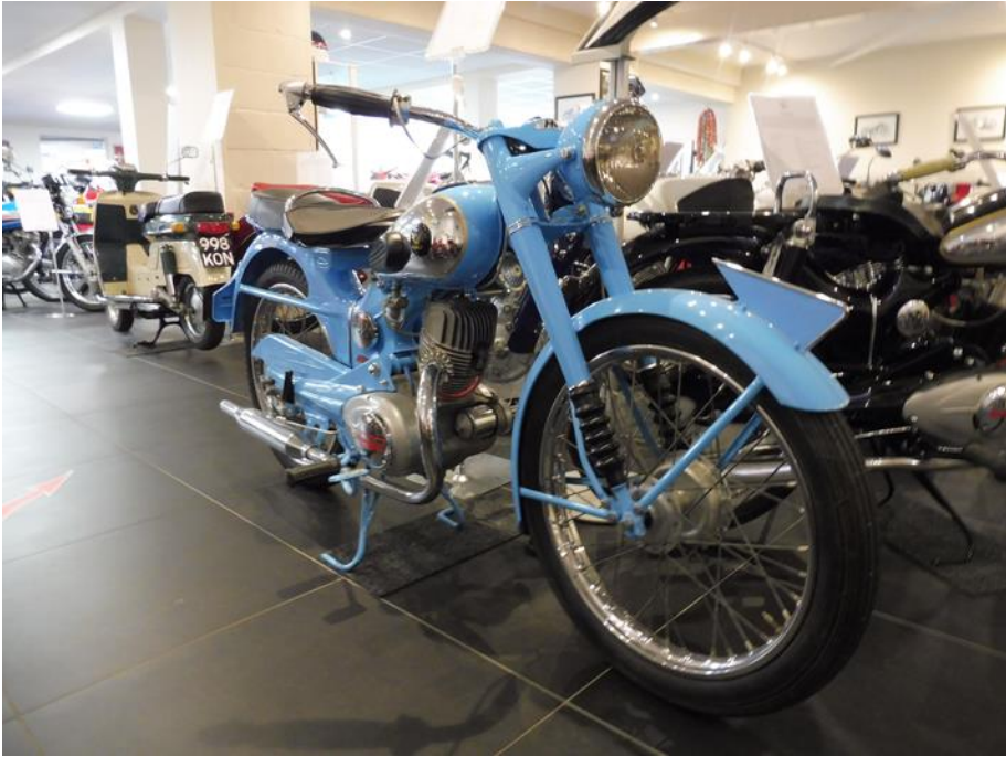
The first Benly (from the Japanese word Benri , meaning convenient ), an 89cc, 3-speed 1954 Benly J-Type from the second year of manufacture. Although based on the NSU Fox, it featured several Honda innovations including the engine attached to the swinging-arm suspension by a see-saw arrangement.
