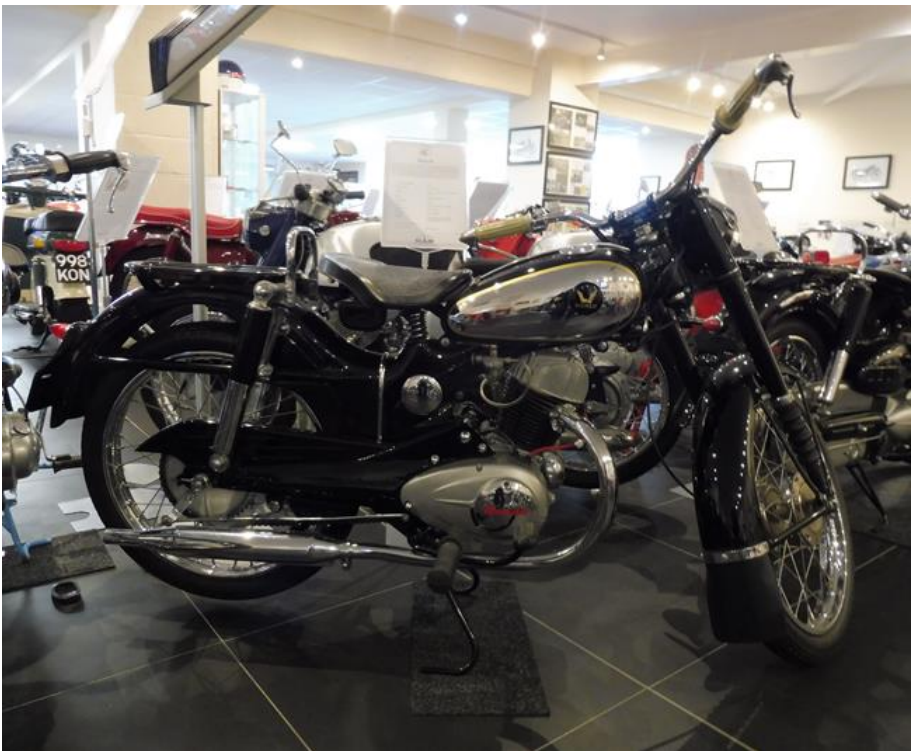
1955 Benly JB – 125cc three-speed, four-stroke. Introduced a year after the 138cc Benly JA to take advantage of a change to the Japanese driving laws which meant that no licence was needed to ride machines up to 125cc.
