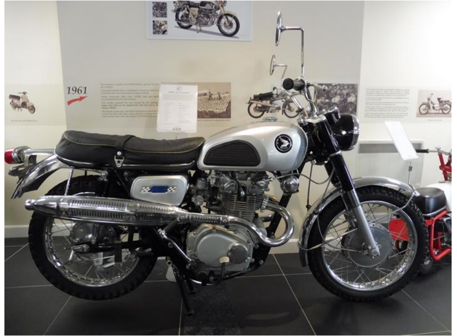
1968 CB450D “Desert Scrambler” – essentially a Black Bomber wearing a beauty kit to help shift large stocks of the rather dull looking standard machine piled up in American showrooms. Comprising a tank, seat, mudguards, upswept exhausts and a few other bits to transform it into what was later the CL range of offroad-styled machines.
