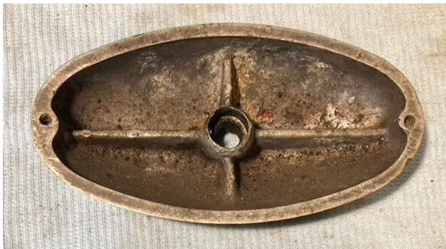
Huntmaster valve cover, this one surprisingly uncracked
