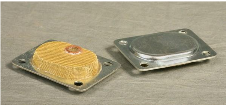
'Pressed tin sump plate'
