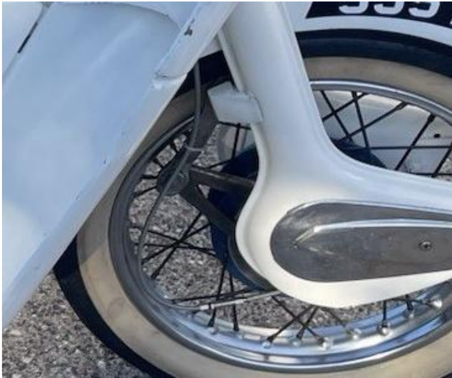
Not easy to see, the brake anchor of an Ariel Leader offered by a private seller . . .
