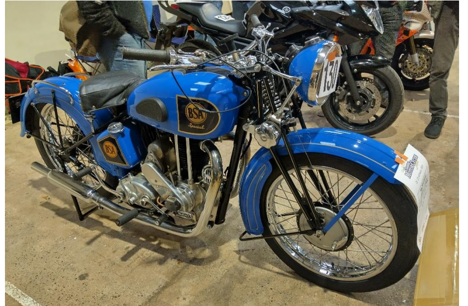
BSA 500cc Special – JAP engine from a 1929 French Terrot fitted in a 1939 BSA WM20 frame left behind at Dunkirk
