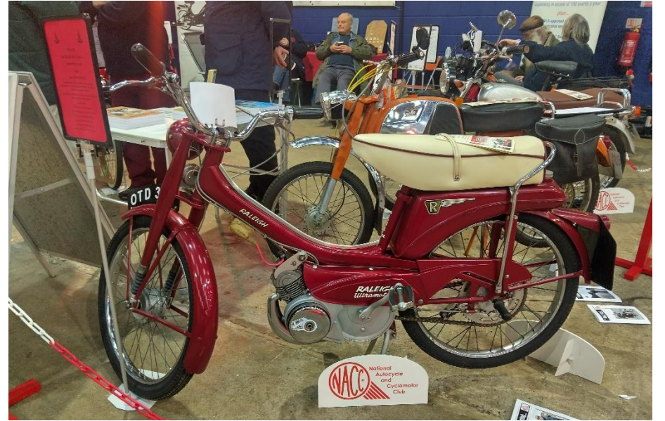
1968 Raleigh Ultramatic RM9+1 – rare dualseat model with more powerful engine and variator transmission
